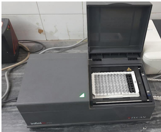
Figure 1: TECAN INFINITE F50 Absorbance Microplate reader for ELISA.
