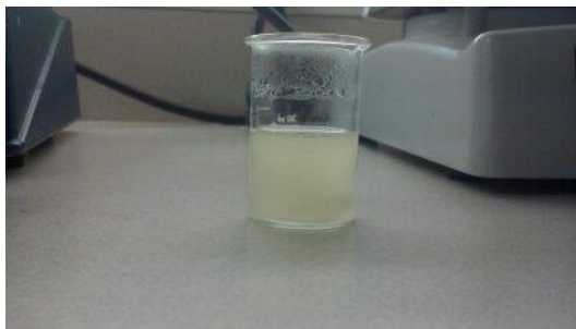
Figure 5: Control mixture of 25 mL NS, pH 7.4, at 37°C with 0.45 g PC (95% ± 5%) melted uniformly throughout.
