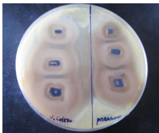
Figure 11: Image of zone inhibition for Vibrio cholerae (left) and Pseudomonas aeruginosa (right) by the specific amount of 50 \mu L, 100 \mu L, and 120 \mu L of Mn_3O_4 loaded CNTs.
