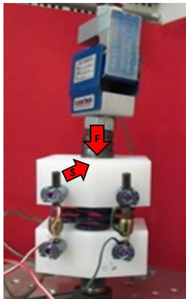
Figure 3: Flexo-compression test configuration and load applied.
