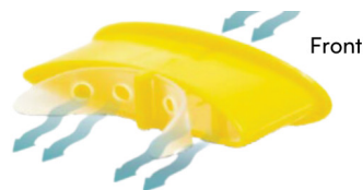
Figure 2a: During inspiration, the ExVent valve is open.
