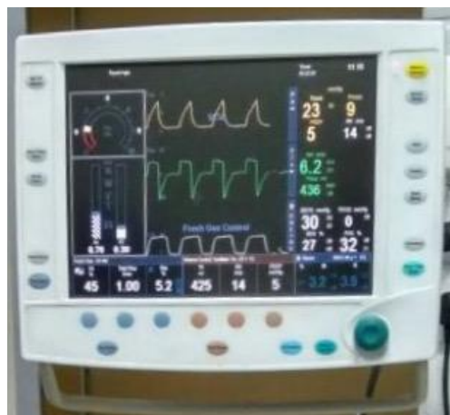
Image 2: Manual fresh gas flow mode.
